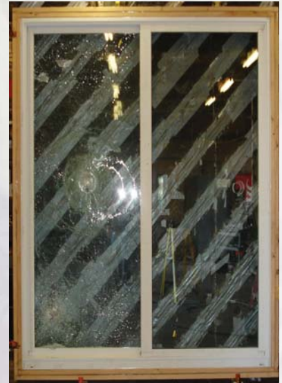
After Impact & Cyclic Pressure Test Specimen Successfully Passes Impact & Cycling Testing
