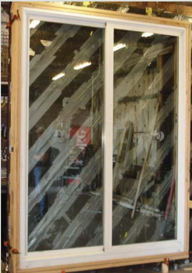
Before Impact & Cyclic Pressure Test Specimen glazed with 1" IG (1/4" clear ann'd x 1/2" Air Space x 3/8" Laminate with 0.090" PVB interlayer
